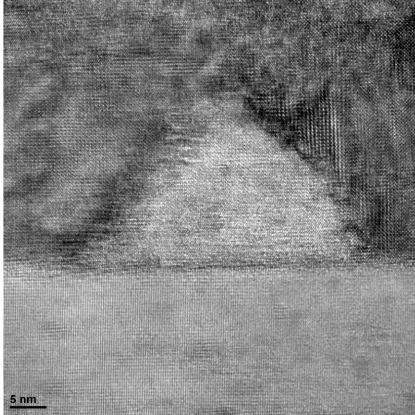
Figure 3.7: HRTEM of a pyramidal pit formed in a thick epitaxial HT-grown VO 2 film on C-sapphire
