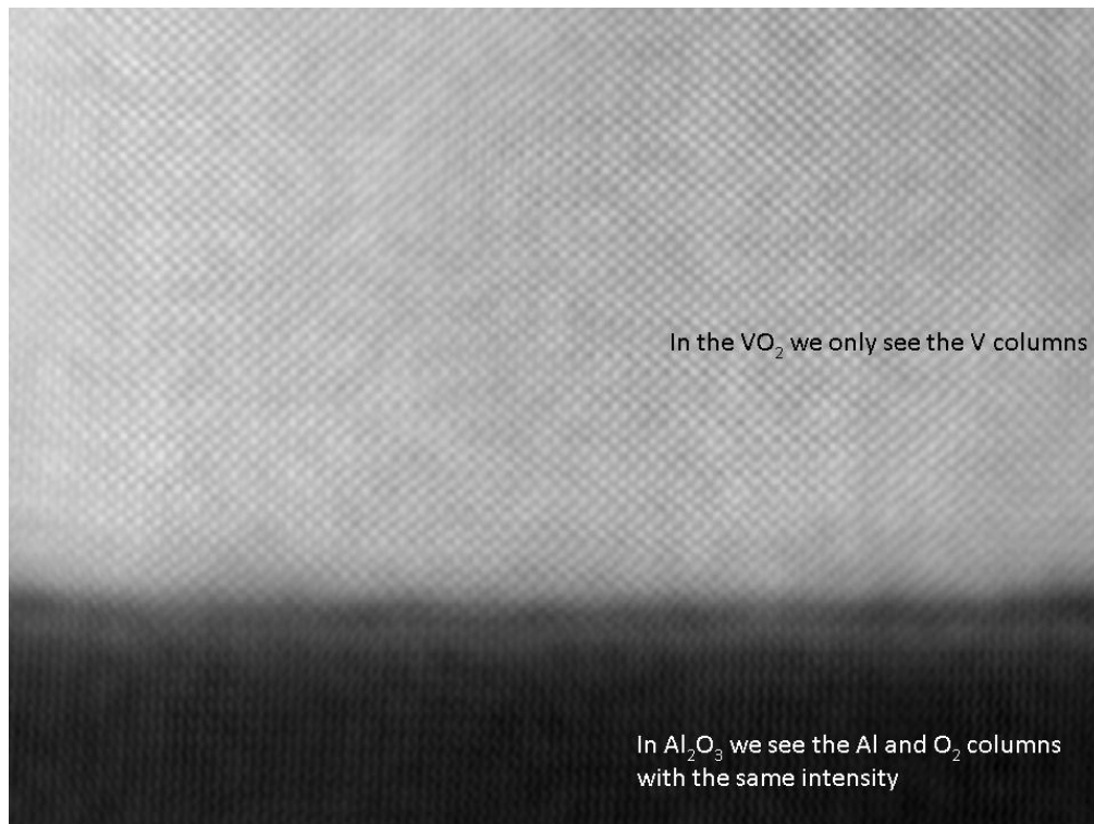
Figure 2.18: Z-contrast Scanning Transmission Electron Microscopy image of the \text{VO}_2 -C-sapphire interface. Courtesy: Dr. Gerd Duscher, Oak Ridge National Laboratory.
