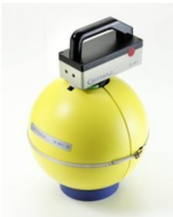
Figure 2.6. An example ICRP 60-inspired "moderator sphere". (Credit: Berthold)
