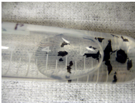
Figure 5-9. Free-standing carbon nanotube films (buckypapers) produced by John Rigueur using the SLED technique. Figure provided by John Rigueur.
