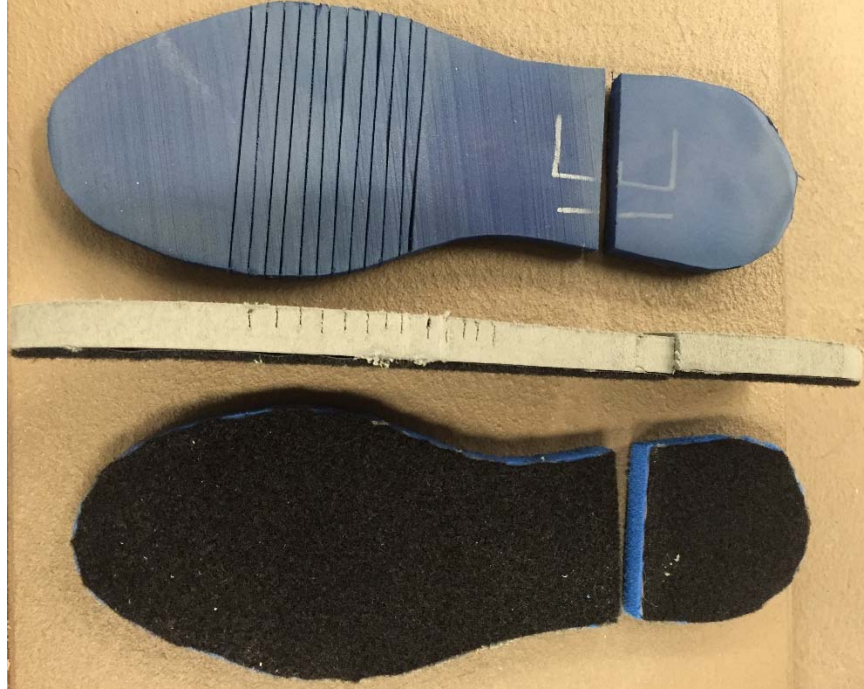
Figure 11: Sole cushioning conditions showing color, thickness, heel-forefoot separation, bending slits, and adhered loop (for hook-and-loop attachment). From top to bottom: Hard forefoot and heel, medium forefoot and heel, soft forefoot and heel.
