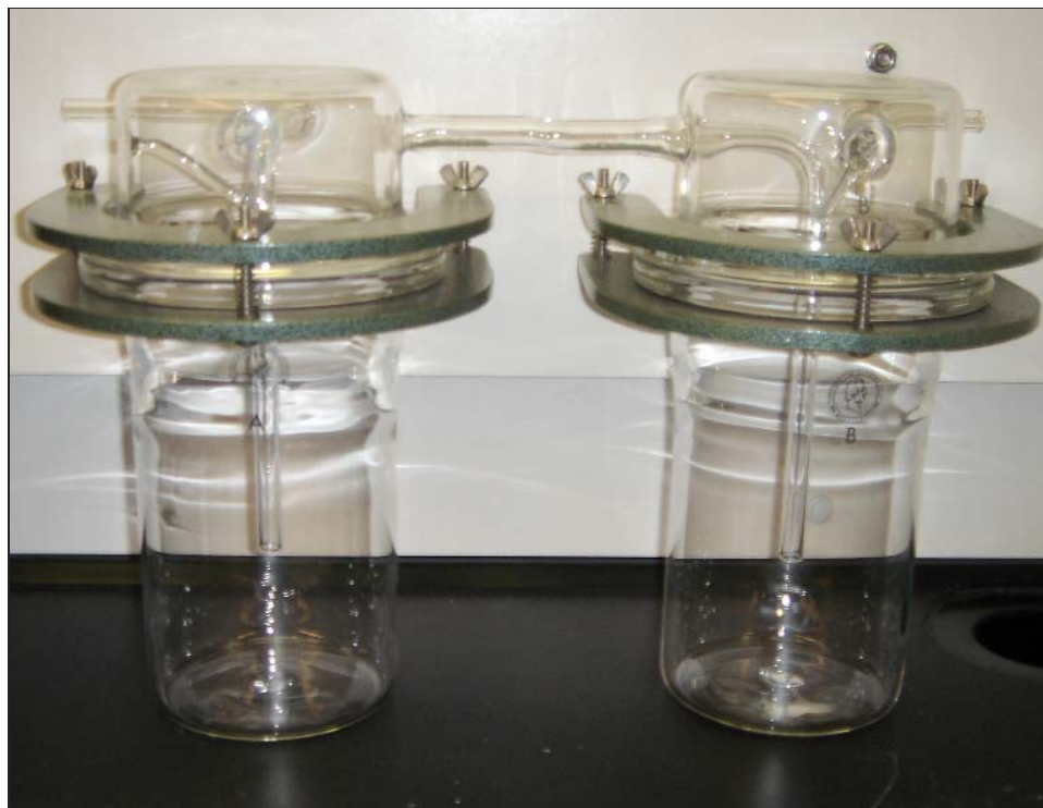
Figure A.13: Picture of custom-built bubbler.
