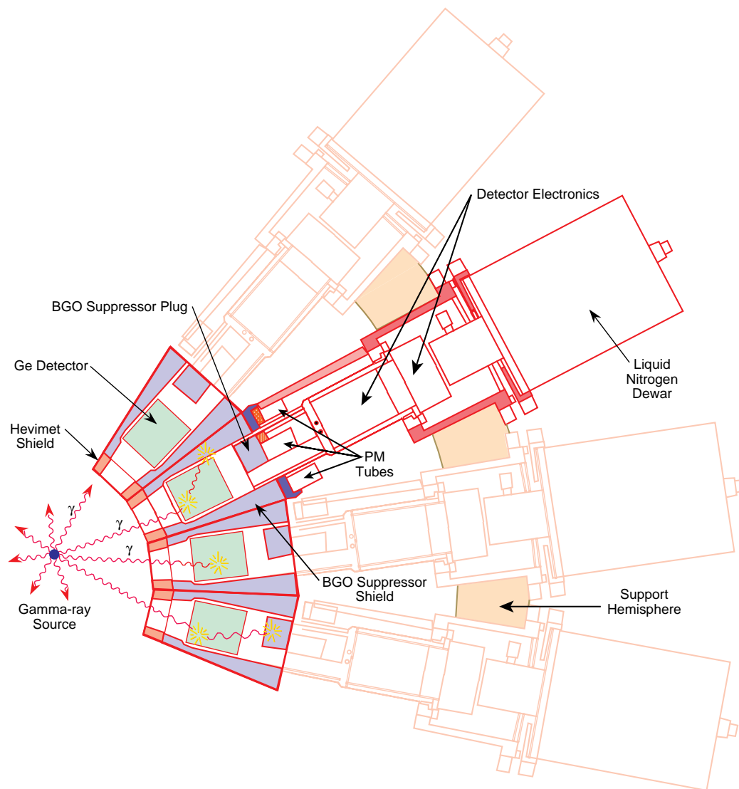
Figure 10: A schematic diagram of a Gammasphere detector module showing the Ge crystal ( \sim 10\text{cm} long), the BGO/photomultiplier suppression system, the housing for the electronic control system and also the liquid-nitrogen dewars used to cool the Ge crystal in order to suppress random thermal signals.
