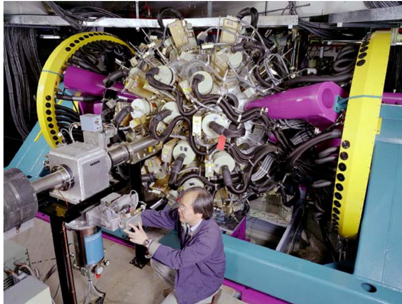
Figure 9: Gammasphere closed and ready for beam. The array is split vertically down the middle so that the system can be pulled apart for access to the source chamber at the center of the sphere.
