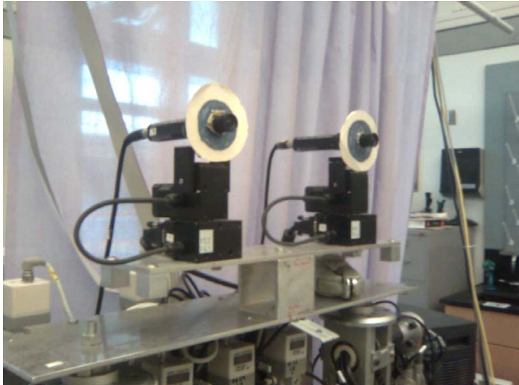
Figure 2: The two camera modules, the lenses and the mounts constitute ISAC's eyes
