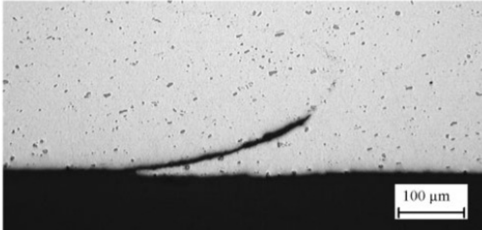
Figure 5: Joint line remnant at the root of the joint line
