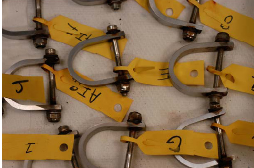
Figure 12: U-bend test samples prior to NaCl testing from Clark
