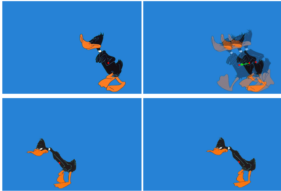
Figure V.10: Illustration of applying a pre-computed velocity vector from an original sequence to a re-sequenced frame. Top left shows a frame in a re-sequenced animation, bottom left shows the next frame in the re-sequenced animation. Top right illustrates the velocity vector computed for the frame in the top left. Bottom right shows the realignment of the character from the second re-sequenced frame. Daffy is TM & © Warner Bros. Entertainment Inc.
