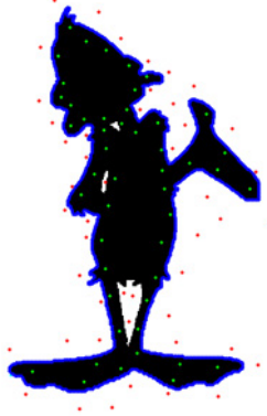
Figure II.13: An example of defining an implicit function to represent a cartoon character from an image. The blue points (densely sampled) are the zero set, the green points are interior points, the red are exterior points. To facilitate viewing these points, the cartoon character’s silhouette is shown instead of the full color frame.
