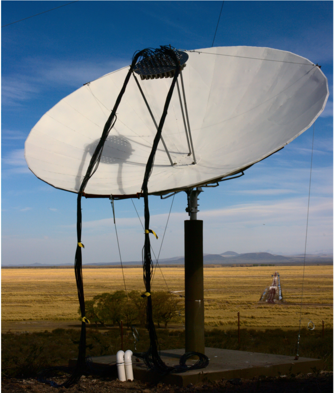
Figure 3.1: The MIDAS telescope at the Pierre Auger Observatory, with the 53-pixel camera mounted at the prime focus of the 5 m diameter parabolic dish reflector. Figure acquired from Williams (2013).
