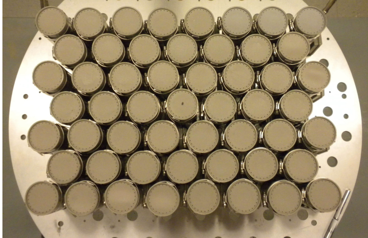
Figure 3.2: Image of the 53-pixel camera at the focus of the MIDAS telescope. Figure acquired from Alvarez-Muiz et al. (2013).
