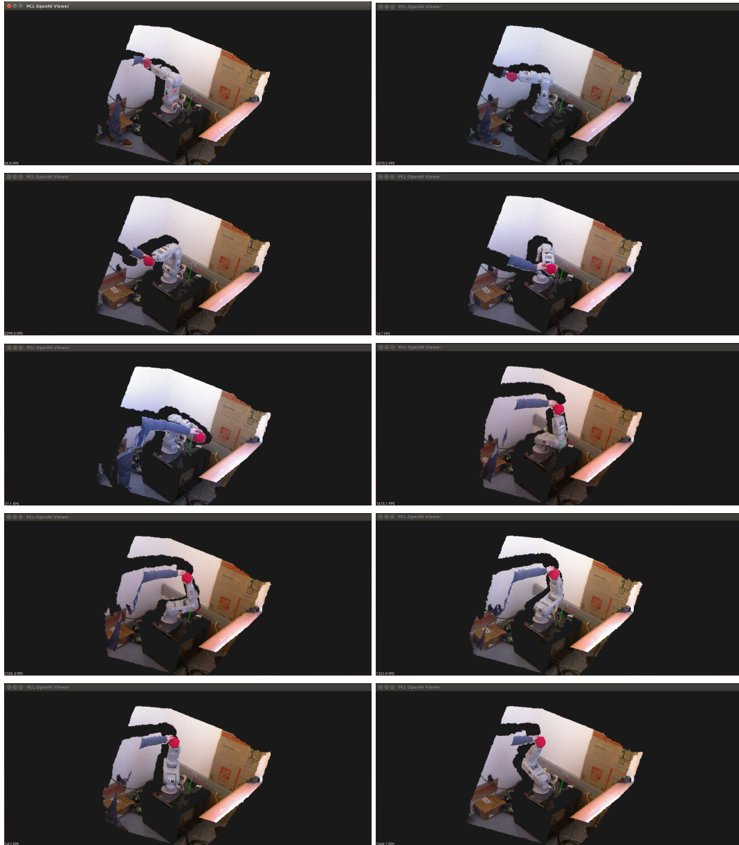
Figure 3.2: Sequence of Movements Used to Calibrate the Robot
