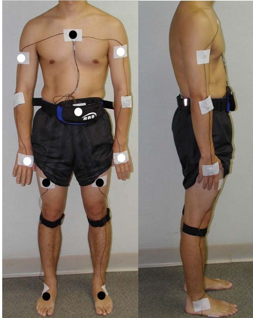
Figure 2: Illustration of IDEEA sensor locations. Sites shown in black represent the original accelerometer sites, while sites in white are the custom sensor sites.
