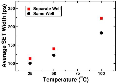
Fig. 5.22: Average SET width measurements as a function of temperature for the separate well and same well 1000-inverter chain target circuits.
