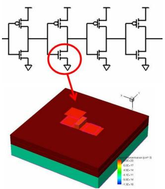
Fig. 4.8: Illustration of the mixed-mode model used for the simulations. The second nMOSFET in a four inverter chain was modeled in 3D TCAD, and the remaining inverters were modeled in SPICE.
