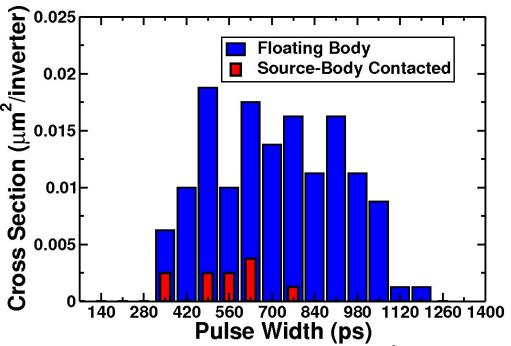
Fig. 4.4: SET pulse width distributions for xenon (LET =  $69 \text{ MeV-cm}^2/\text{mg}$ , Fluence =  $4 \times 10^8 \text{ particles/cm}^2$ ).
