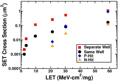
Fig. 6.4: SET cross section for the different 65-nm test structures. Note that the threshold LET for the "P-hit" and "N-hit" circuits are much larger than that for the inverter chain circuits.
