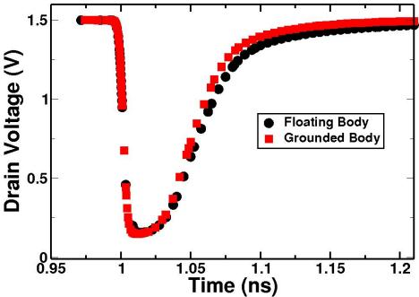
Fig. 4.10: Simulated SET pulse widths at the struck node for an LET of 40 MeV-cm<sup>2</sup>/mg for the non-body contacted device and the body contacted device. The ion strike location in this simulation was the center of the gate.
