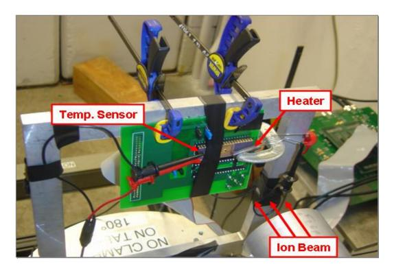
Fig. 5.8: Photograph of the test setup for all of the elevated temperature testing performed in this work.
