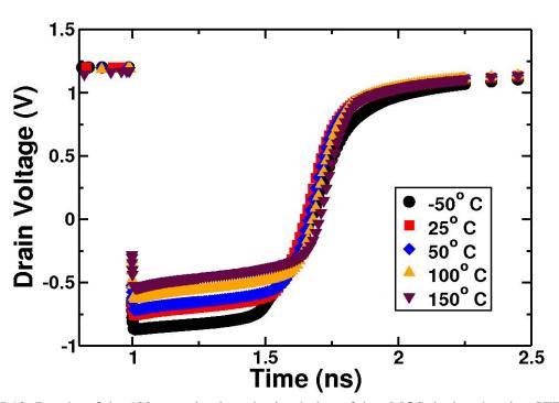
Fig. 5.12: Results of the 130-nm mixed-mode simulation of the nMOS device showing SET pulses on the struck node.
