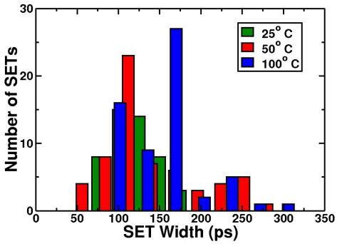
Fig. 6.7: Measured SET pulse width distribution for the "N-hit" circuit. Due primarily to the small number of SETs measured, changes in the SET width distribution are difficult to observe.
