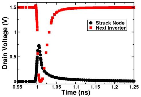
Fig. 4.13: Simulated SET pulse width for a strike on the pMOS device with an LET of 100 MeV-cm<sup>2</sup>/mg.
