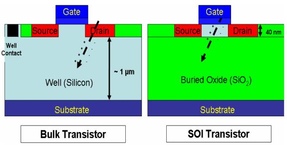
Fig. 2.4: Cross-section of a bulk and SOI transistor
