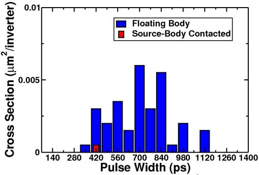
Fig. 4.2: SET pulse width distributions for argon (LET =  $14 \text{ MeV-cm}^2/\text{mg}$ , Fluence =  $1 \times 10^9$  particles/cm<sup>2</sup>). Note that not only are the pulse widths shorter for the circuit with source-body contacts, the total the number of counts is also significantly less.
