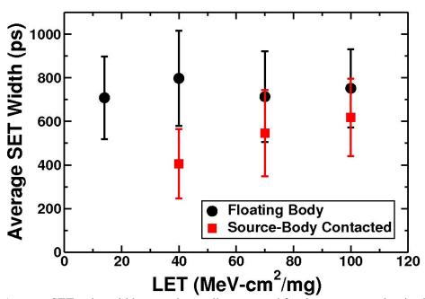
Fig. 4.6: Average SET pulse widths experimentally measured for the two target circuits. The error bars represent one standard deviation from the average.
