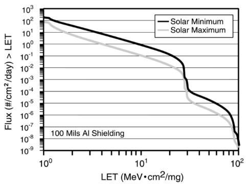
Fig. 2.2: Flux of energetic particles in space as a function of linear energy transfer (LET) [Xaps-06]
