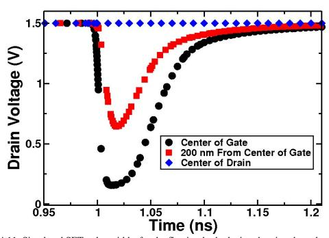
Fig. 4.11: Simulated SET pulse widths for the floating-body device showing the pulse width dependence on the ion strike location. As the strike location moves away from the center of the gate, the SET pulses become smaller. An ion strike at the center of the drain creates no SET.
