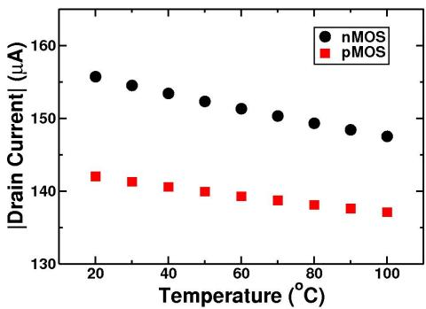
Fig. 5.26: Simulated drain current as a function of temperature for the 65-nm nMOS and pMOS devices used in the inverter chain target circuit.
