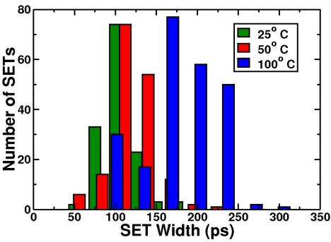
Fig. 5.20: Measured SET pulse width distribution for the same well inverter chain circuit. Note that as the temperature increases the distribution shifts to the longer SET widths
