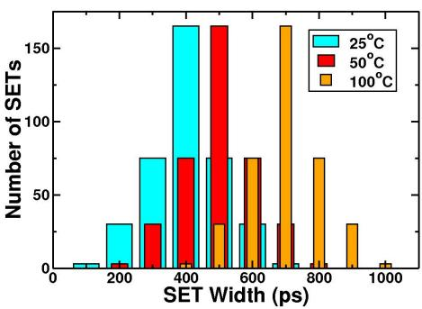
Fig. 5.19: Plots of a possible original distribution of SETs without pulse broadening for  $25^{\circ}$  C,  $50^{\circ}$  C, and  $100^{\circ}$  C.
