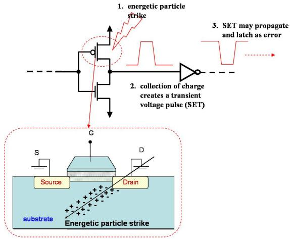
Fig. 2.5: Figure detailing how charge collected at a circuit node can create a transient signal that can propagate through a logic chain [Nara-08].
