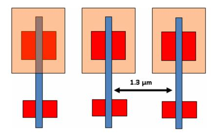
Fig. 3.12: Illustration of the layout of the separate well inverter chain target circuit.
