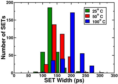
Fig. 6.6: Measured SET pulse width distribution for the "P-hit" circuit. Note that as the temperature increases the distribution clearly shifts to the longer SET widths.
