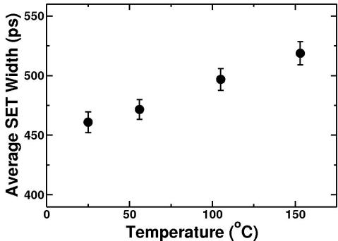
Fig. 5.9: Average SET pulse width for the elevated temperature testing of the 130-nm test circuits.
