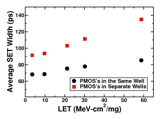
Fig. 3.13: Average measured SET width versus LET for the separate well and same well test 65-nm test structures.
