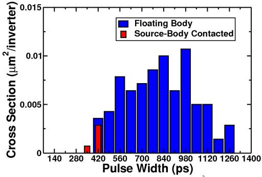
Fig. 4.3: SET pulse width distributions for krypton (LET =  $40 \text{ MeV-cm}^2/\text{mg}$ , Fluence =  $7x10^8$  particles/cm<sup>2</sup>).
