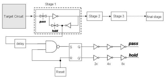
Fig. 2.10: Diagram of the complete self-triggering autonomous SET test structure with reset [Nara-06]
