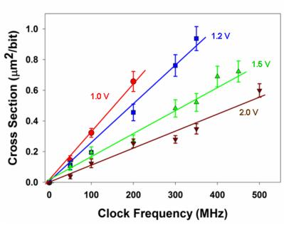
Fig. 2.7: Cross-section versus frequency for several different operating voltages [Gadl-07]
