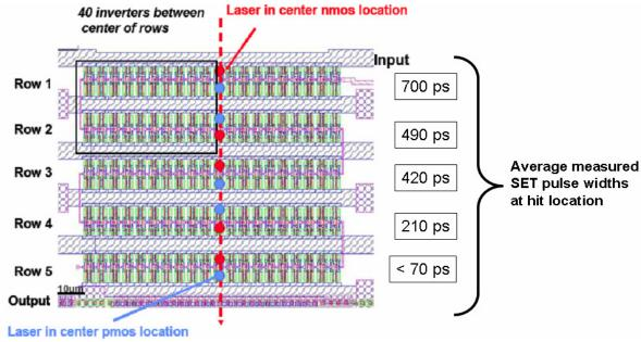
Fig. 4.1: Average measured SET widths for various strike locations in the inverter chain target circuit for the floating-body FDSOI test structure.
