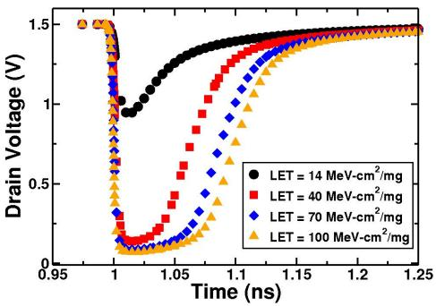
Fig. 4.12: Simulated SET pulse width distributions for strikes on the nMOS device for the ions used in testing.
