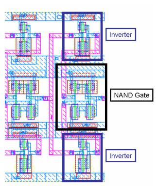
Fig. 6.3: Layout of two of the blocks of "N-hit" target circuit. The spacing between the two inverters needs to be large enough to ensure that an ion can not induce an SET on both at the same time.
