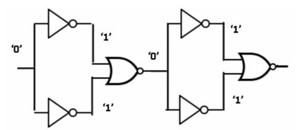
Fig. 6.2: Schematic of two of the blocks of "P-hit" target circuit. The target circuit used in this work consisted of four linear chains of 100 of these combinational logic blocks "OR"-ed together to form a single output.
