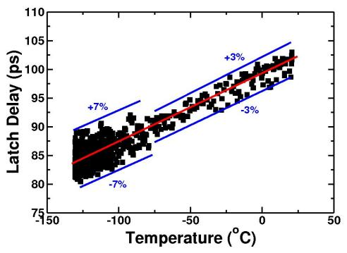
Fig. 5.1: 130-nm stage delay as a function of temperature.
