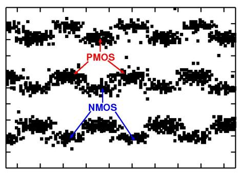
Fig. 3.15: SET error map of the separate well target circuit taken at the microbeam facility
