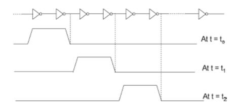
Fig. 2.8: Illustration detailing how an SET with a width of two inverters delays propagates through an inverter chain [Nara-06]
