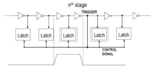
Fig. 2.9: An illustration of the technique used in the autonomous SET measurement circuit to capture pulse widths [Nara-06]
