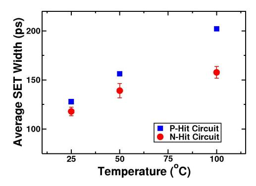
Fig. 6.5: Average SET width as a function of temperature for the "N-hit" and "P-hit" circuits.
