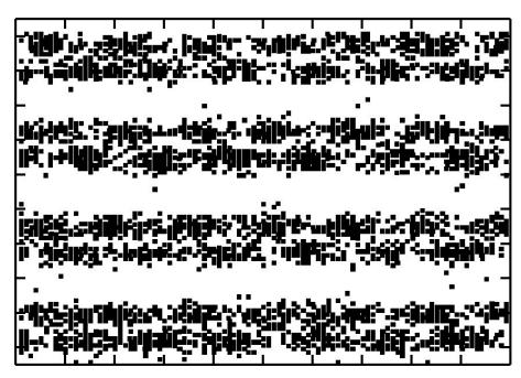
Fig. 3.16: SET error map of the same well target circuit taken at the microbeam facility.
