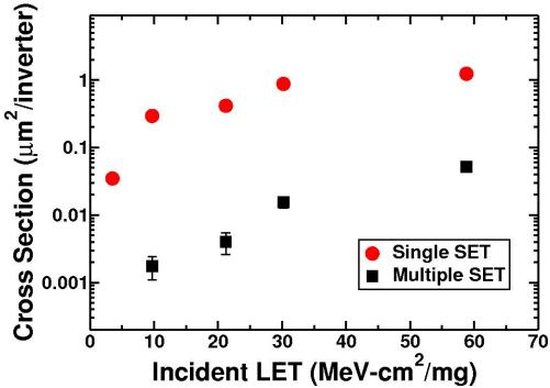
Fig. 3.18: Comparison of the multiple SET cross-section to the single SET cross-section for the separate well target circuit.
