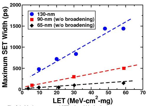
Fig. 3.6: Maximum generated SET pulse widths for the three test structures.
