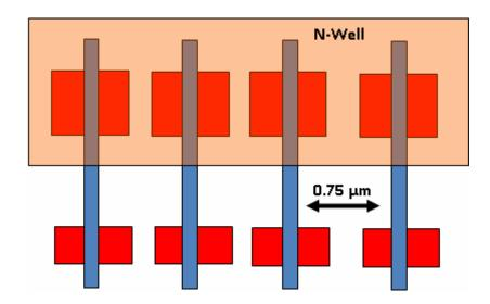
Fig. 3.11: Illustration of the layout of the same well inverter chain target circuit.
