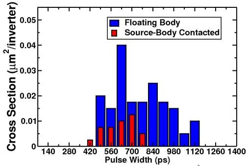
Fig. 4.5: SET pulse width distributions for bismuth (LET =  $100 \text{ MeV-cm}^2/\text{mg}$ , Fluence =  $2 \times 10^8 \text{ particles/cm}^2$ ).
