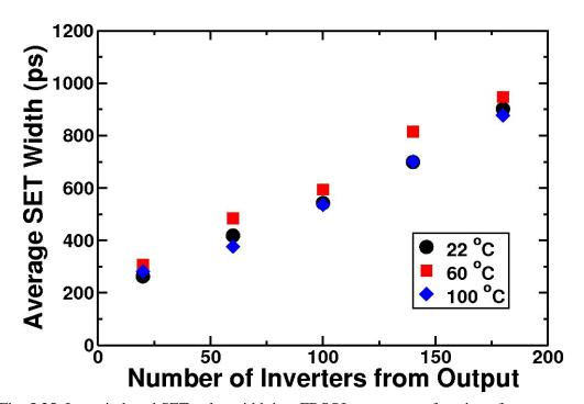
Fig. 5.25: Laser induced SET pulse width in a FDSOI process as a function of temperature.
