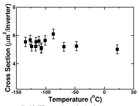
Fig. 5.3: SET cross-section as a function of temperature.
