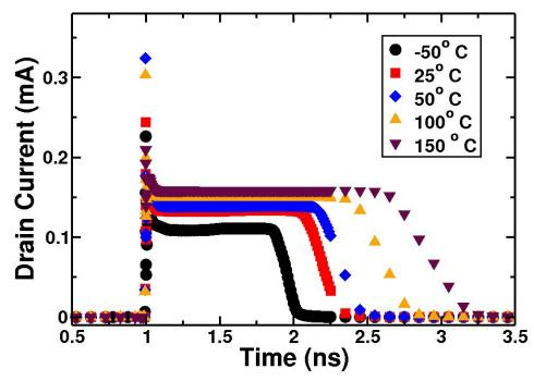
Fig. 5.13: Results of the 130-nm mixed mode simulation showing the drain current on the struck node of the pMOS device for five temperatures.
