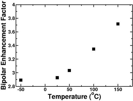
Fig 5.15: Bipolar enhancement factor plotted as a function of temperature.
