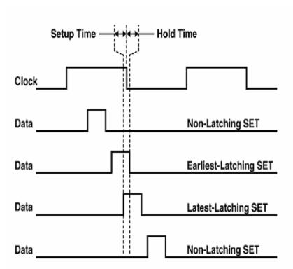
Fig. 2.6: SETs arriving at the latching edge of a clock can be recorded as incorrect bits [Mavi-02].
