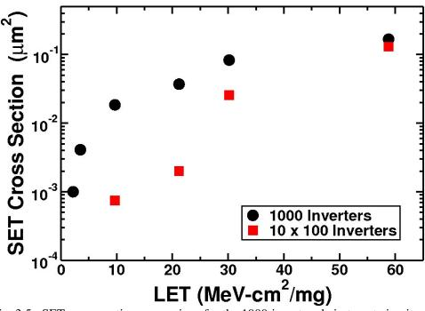
Fig. 3.5: SET cross-section comparison for the 1000-inverter chain target circuit and the 10x100 inverter chain target circuit.
