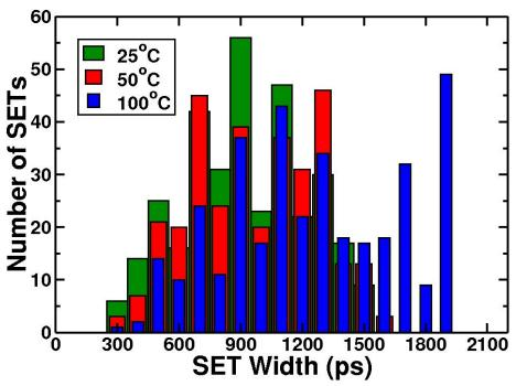
Fig. 5.16: 90-nm bulk SET pulse width distribution for xenon (LET=52 MeV-cm²/mg) at temperatures of 25° C, 50° C, and 100° C. At 100° C, some of the SETs were longer than the measurement limit of the test circuit.
