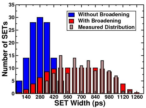
Fig. 4.7: Plots of a possible original distribution of SETs without pulse broadening, the distribution obtained by convolution of the broadening-caused effects, and the actual measured SET events.
