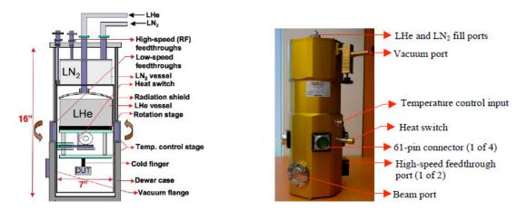
Fig. 5.2: Illustration and photograph of the cryogenic test system used in this work.
