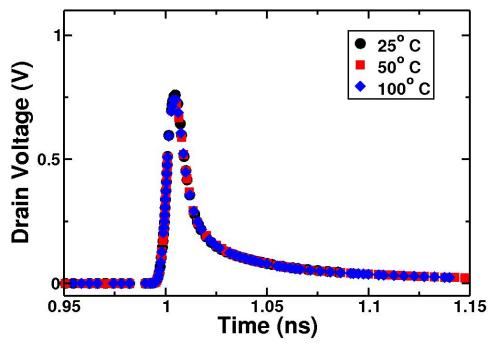
Fig. 5.24: Results of the 180-nm FDSOI mixed mode simulation for the pMOS device showing SET pulses on the struck node.
