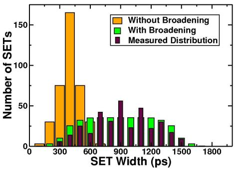
Fig. 5.18: Plots of a possible original distribution at 25° C of SETs without pulse broadening, the distribution obtained by convolution of the broadening-caused effects, and the actual measured SET events.
