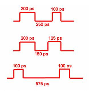
Fig. 3.17: Examples of some of the multiple SET events measured during heavy ion testing of the separate well circuit.
