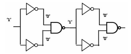
Fig. 6.1: Schematic of two of the blocks of "N-hit" target circuit. The target circuit used in this work consisted of four linear chains of 100 of these combinational logic blocks "OR"-ed together to form a single output.
