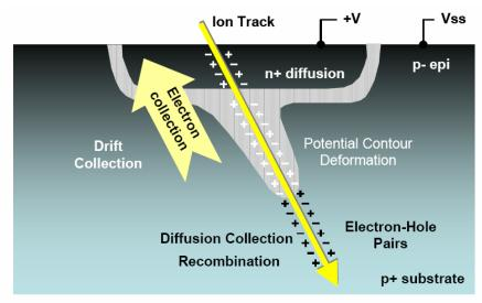
Fig. 2.3: Illustration showing the different charge collection mechanisms during a single event [Baum-05]
