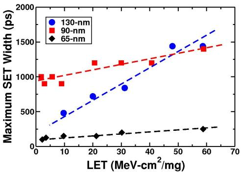
Fig. 3.1: Maximum SET widths measured in the 130-nm, 90-nm, and 65-nm test structures
