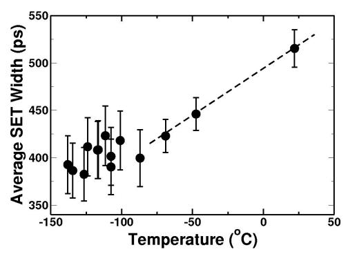
Fig. 5.7: Average SET pulse width for the cold temperature testing.
