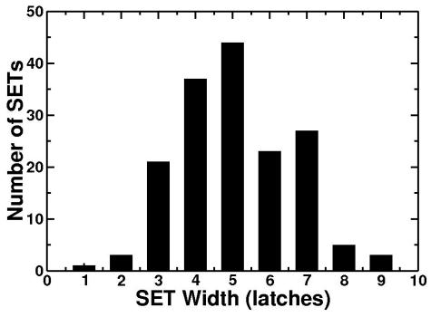
Fig. 5.4: Measured SET pulse width histogram at room temperature. The histograms (in units of latch delays) were similar for all temperatures.
