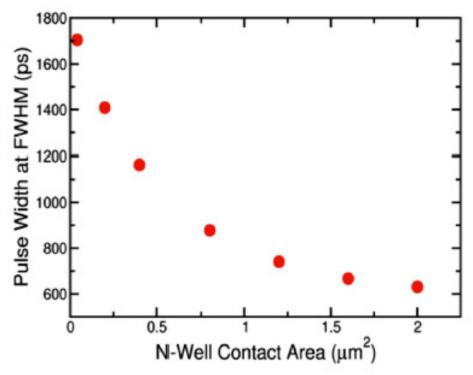
Fig. 3.8: Simulation Results by Amusan et al. showing how the well contact size can affect SET pulse widths [Amus-07].
