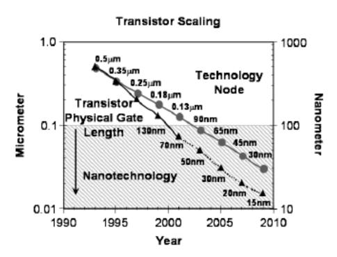
Fig. 2.1: A plot from Intel [Chau-05] showing how the physical gate length of a transistor has continued to shrink over the past two decades.
