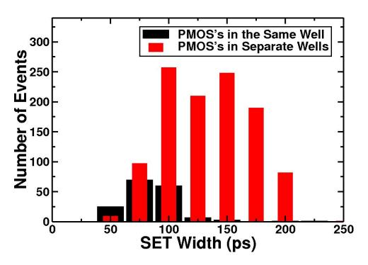
Fig. 3.14: Histogram of the measured SETs for the two 65-nm structures for an LET of 60 MeV-cm<sup>2</sup>/mg.
