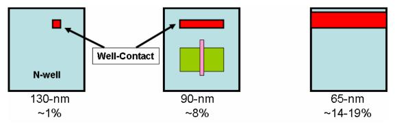
Fig. 3.9: Illustration of the well contacting scheme used for each of the test structures.
