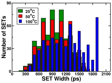
Fig. 5.17: 90-nm bulk SET pulse width distribution for xenon at an incident angle of 50° (effective LET=81 MeV-cm²/mg) at temperatures of 25° C, 50° C, and 100° C.
