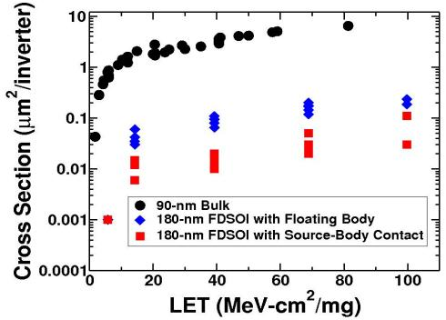
Fig. 4.14: Comparison of bulk and SOI SET cross-sections
