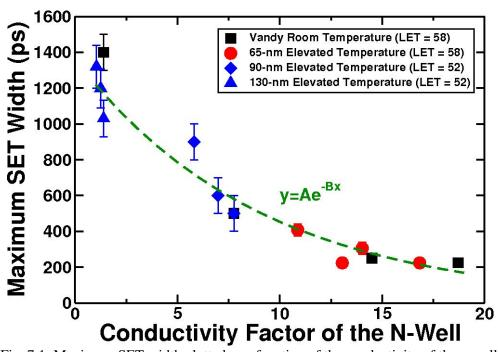
Fig. 7.1: Maximum SET width plotted as a function of the conductivity of the n-well.
