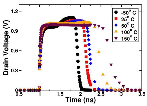
Fig. 5.11: Results of the 130-nm mixed-mode simulation of the pMOS device showing SET pulses on the struck node for five temperatures.
