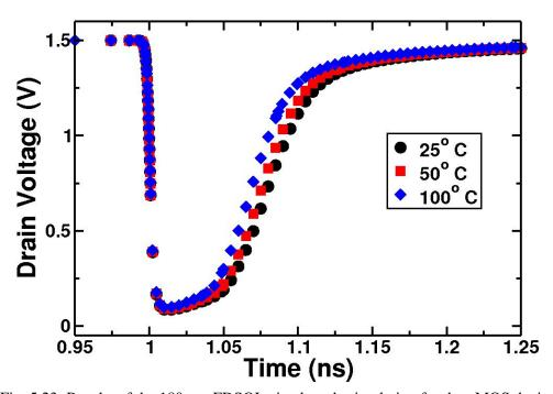
Fig. 5.23: Results of the 180-nm FDSOI mixed mode simulation for the nMOS device showing SET pulses on the struck node for 25° C, 50° C, and 100° C.
