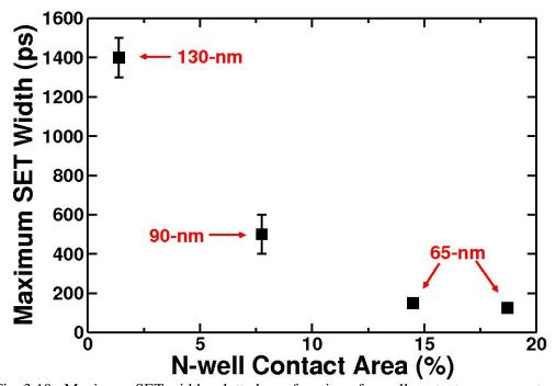
Fig. 3.10: Maximum SET widths plotted as a function of n-well contact area percentage.
