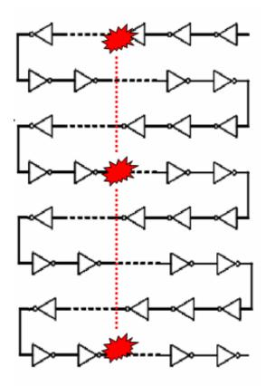
Fig. 3.2: Schematic of the 1000-inverter chain target circuit in the 90-nm test structure.
