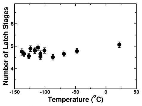
Fig. 5.6: Average SET pulse width in units of latch delays.
