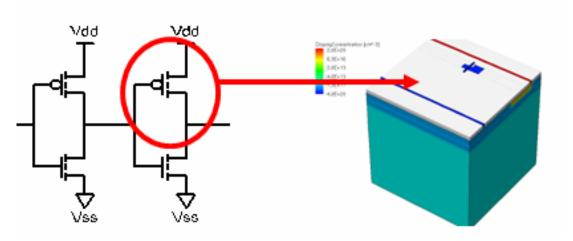
Fig 5.10: A 130-nm TCAD model used to study the effect of temperature on SET pulse widths using a mixed mode simulation. For the 130-nm bulk device, either the off state pMOS or nMOS device was modeled in 3D TCAD.
