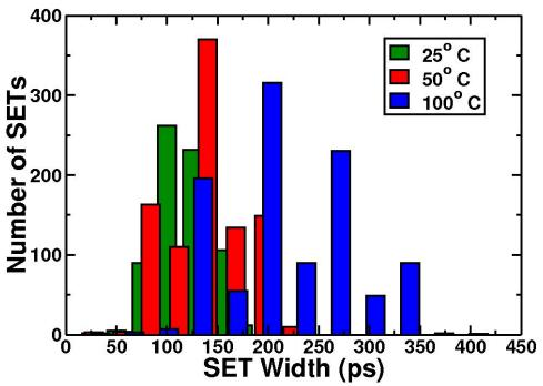
Fig. 5.21: Measured SET pulse width distribution for the separate well inverter chain circuit.
