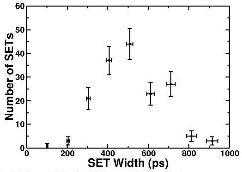
Fig. 5.5: Measured SET pulse width histogram (with error bars) at room temperature.
