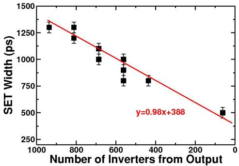
Fig. 3.3: Laser results from the 90-nm SET test structure. Using the same laser energy to strike different locations in the inverter chain shows that as the SET propagates through it widens at a rate of nearly 1 ps/inverter.
