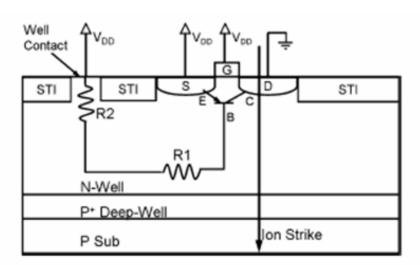
Fig. 3.7: Illustration of a parasitic bipolar transistor in a pMOS device [Olso-07]
