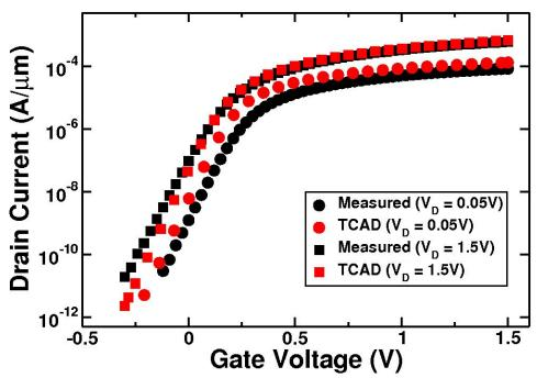
Fig. 4.9: Comparison of measured and simulated I-V curves for a device in this technology.
