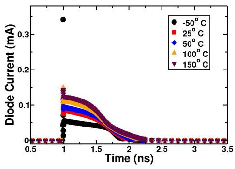
Fig. 5.14: Results of the 130-nm mixed mode simulation showing the current on the struck node of the p-diode for five temperatures.
