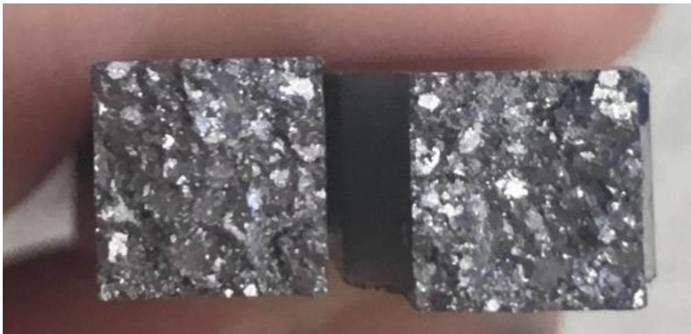
Figure 6. Fracture surface of tensile bar sample A
