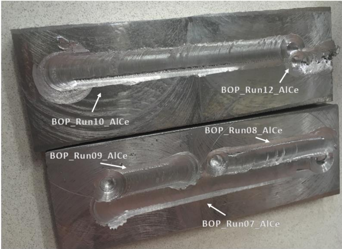
Figure 35. BOP Welding, runs 07-12
