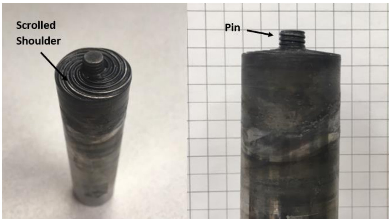
Figure 4. FSW tool with convex scrolled shoulder and threaded cylindrical pin
