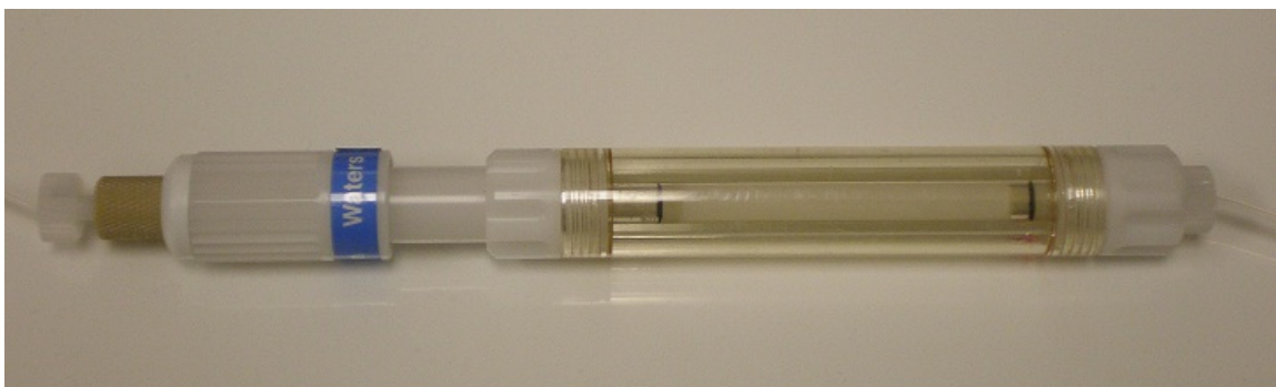
Figure 4-2: AP Minicolumn packed with functionalized porasil particles.
