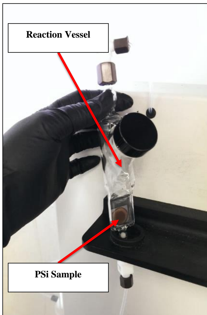
Figure 3.1. Custom reaction vessel for the in situ synthesis of PNA on PSi films.
