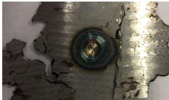
Figure 5.9- FSSW weld region intact with failure in the parent meteorite material
