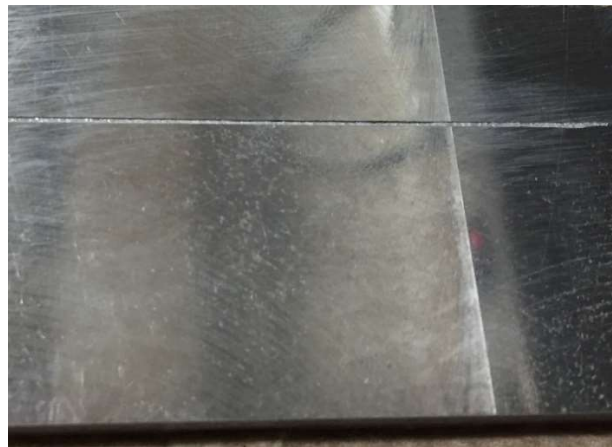
Figure 4.3- UAM 6061 as received from manufacturer, showing milled surface finish and evidence of a tape line.
