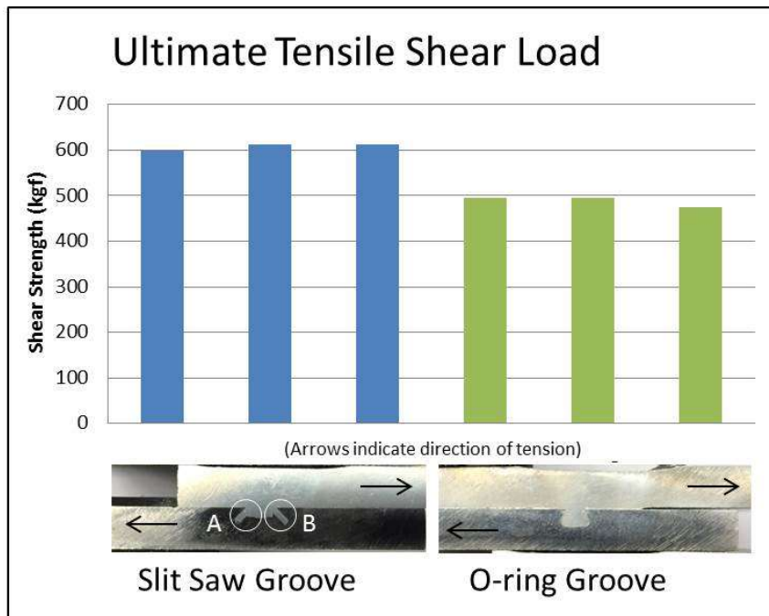
Figure 6.4 Experimental results of FSE for two groove types
