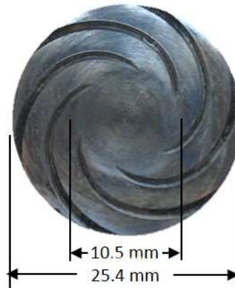
Figure 8.2. Pinless FSSW tool with a spherically tapered shoulder.
