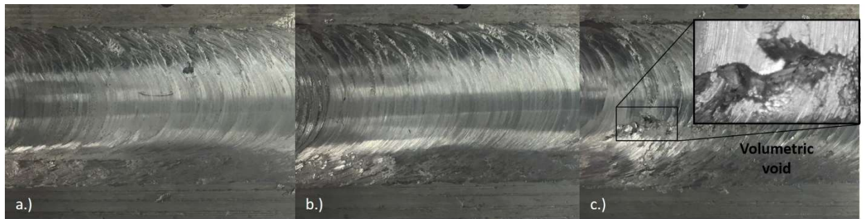
Figure 7.4 Surface Finish of FSE joints at 50.8 mm/min.
