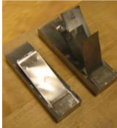
Figure 3.1 Ultrasonic Additively Manufactured Aluminum showing consolidated region created from individual thin sheets.(Graff, Short, and Norfolk)
