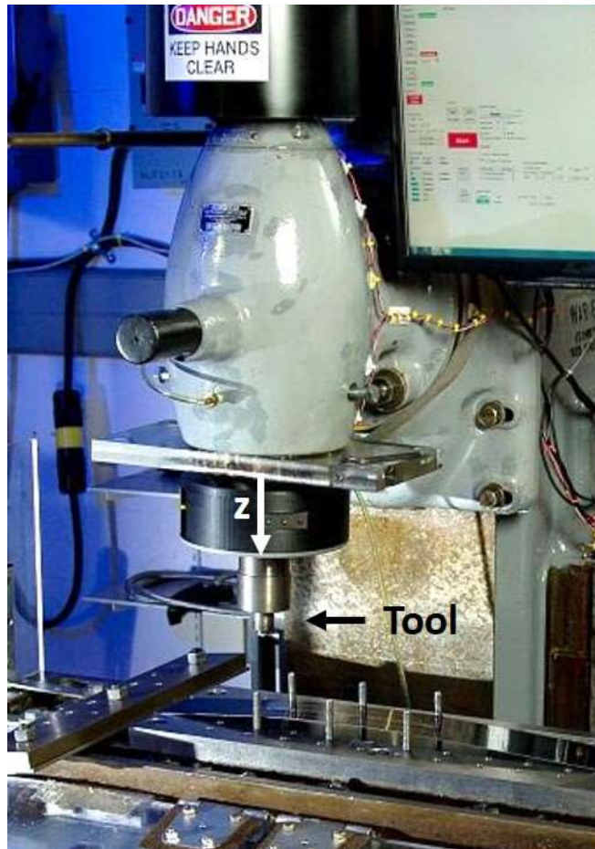
Figure 5.6- Friction Stir Spot Welding Machine
