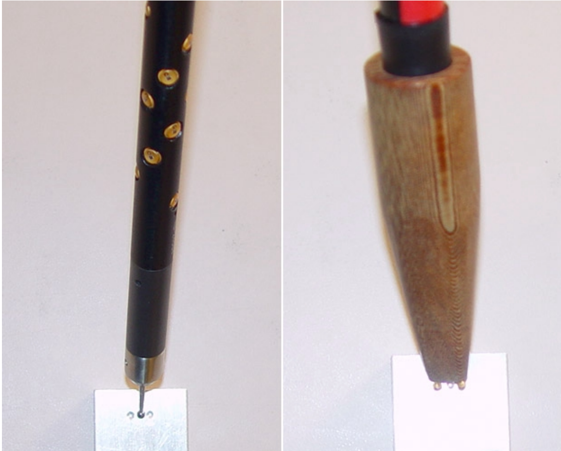
Figure 6.4: The process used to calibrate the tracked cortical stimulator. A standard localizing probe is placed in the center divot of the calibration block and its position is recorded (left). The tips of the stimulator are then placed in the outside divots in order to calibrate the device.
