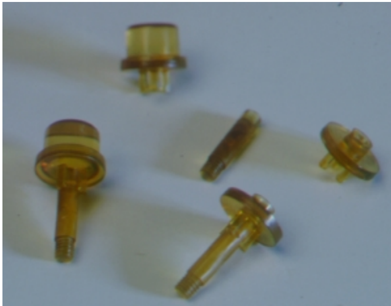
Figure 2.3: Fiducial marker components, showing imaging marker, localizing cap, and screw-in post.
