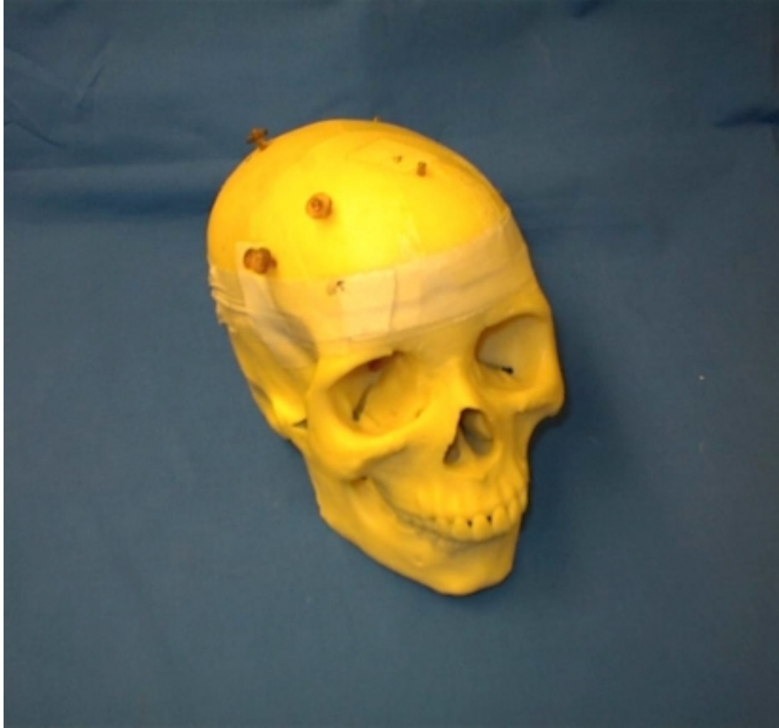
Figure 5.6: Skull phantom showing an imaging marker, localizing cap, and screw-in post.
