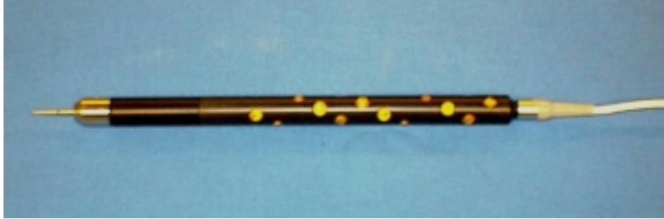
Figure 2.2: Surgical probe with IREDs.
