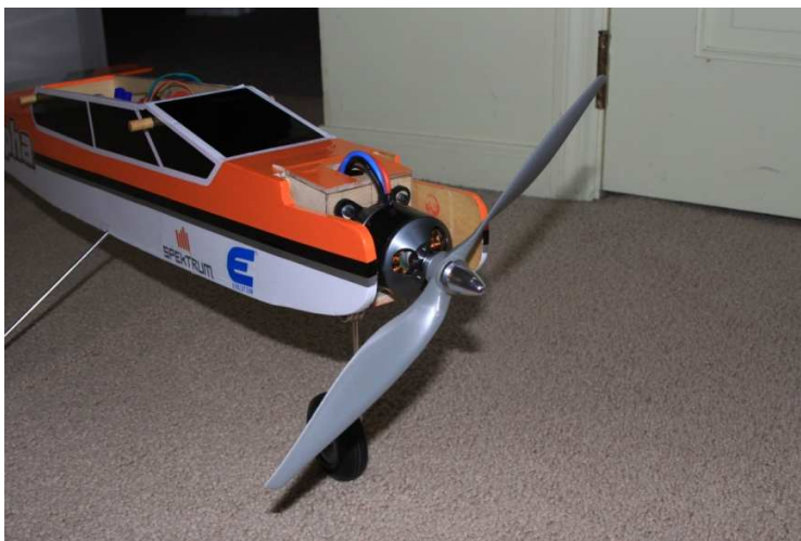
Figure 32 - The upgraded, electric power modification on the Alpha 40
