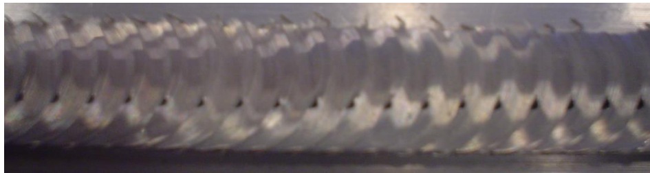
Figure 35: Repeating Surface Defect Caused by Wide Weave Radii [101]
