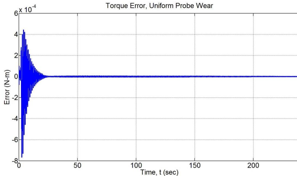
Figure 110: Torque Error While Simulating Uniform Probe Wear
