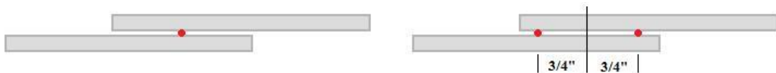
Figure 56: Two Sealant Applications Evaluated by Li et al. [160]: Welding Through Sealant (left) and Welding Between Sealant (right)
