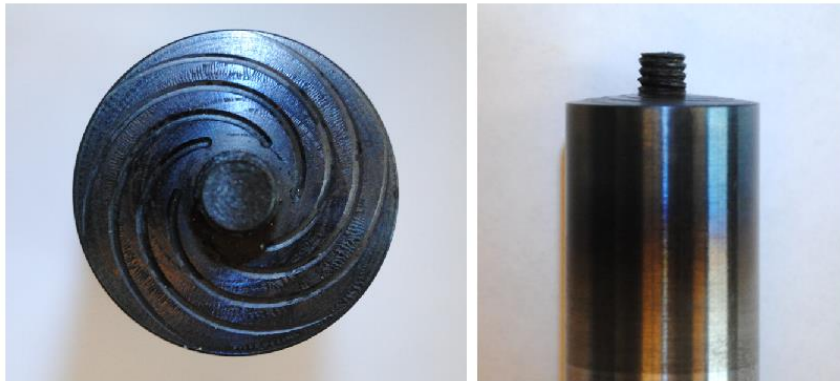
Figure 26: Spherical Scrolled-Shoulder Tool with Threaded Probe [45, 46]
