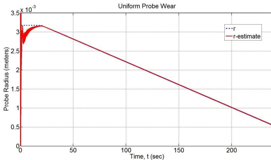
Figure 109: Estimation of Uniform Probe Wear
