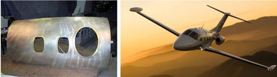
Figure 54: Eclipse 500 Very Light Jet; Completed RH Cabin Assembly (Left) [149], In Flight (Right) [151]
