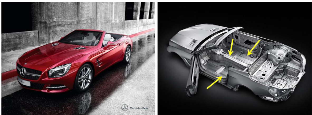
Figure 50: Mercedes SL with Friction Stir Welded Center Tunnel and Floor Panels [137]
