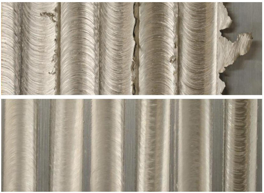
Figure 40: Flat Weld without Torque (or Current) Control (Top); Controlled Weld with 6 mm Rise (Bottom); Image adapted from [46]
