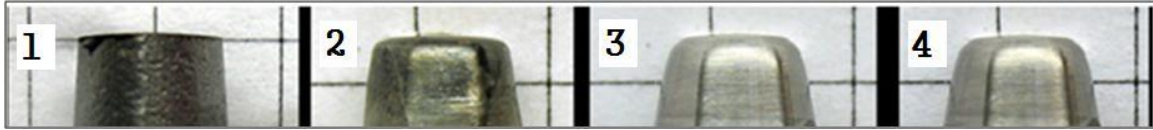
Figure 101: Progressive Tool Wear on MMC at 2000 rpm, 7 IPM; (1) New Probe, (2) 8 Inches of Weld, (3) 16 Inches of Weld, (4) 24 Inches of Weld
