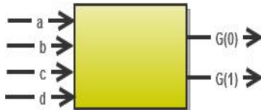
Figure 19: Black-box representation of a combinational circuit
