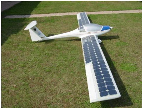
Figure 5: An example of a UAV powered by solar energy. The solar energy drives motors which are connected to propellers in order to generate thrust (La Franchi, 2007).
