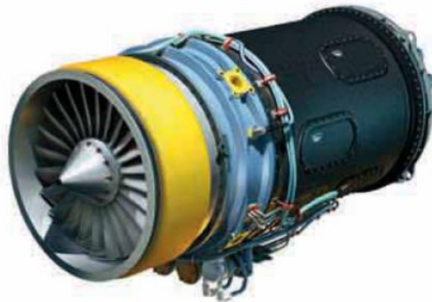
Figure 18: Picture of the Rolls-Royce AE 3007 turbofan engine used in the RQ-4A Global Hawk (Rolls-Royce, 2006).
