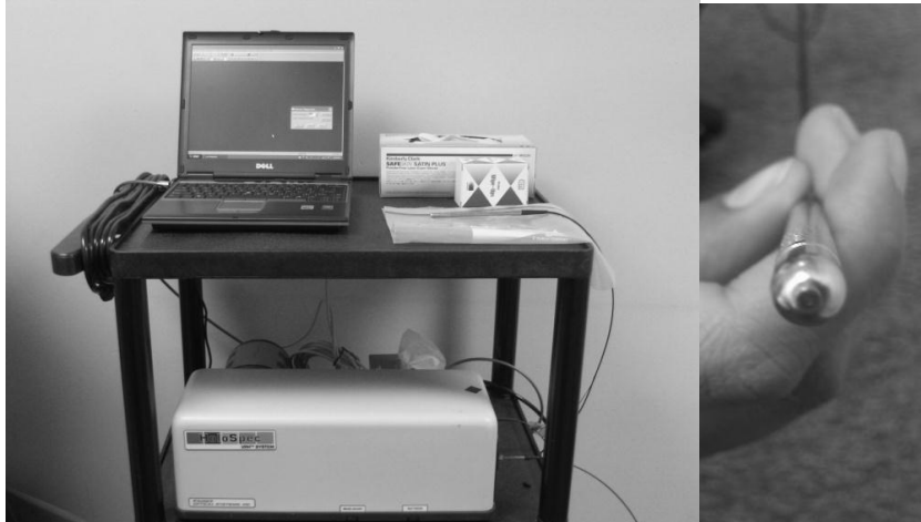
Figure A1.1. Picture of RS system used for in vivo measurements (left) and close-up of Raman probe (right).
