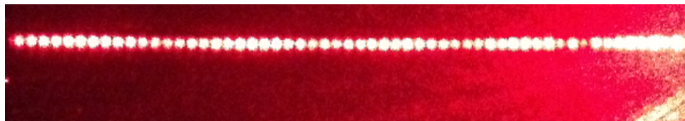
Figure II.6: Interference fringes produced in a forward scattering configuration.
