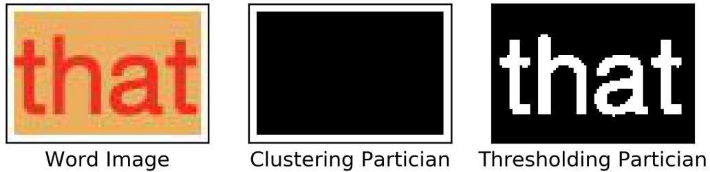
Figure 4.10: How an image snippet of a red and orange-yellow word with a white border is partitioned by the clustering and thresholding approaches.
