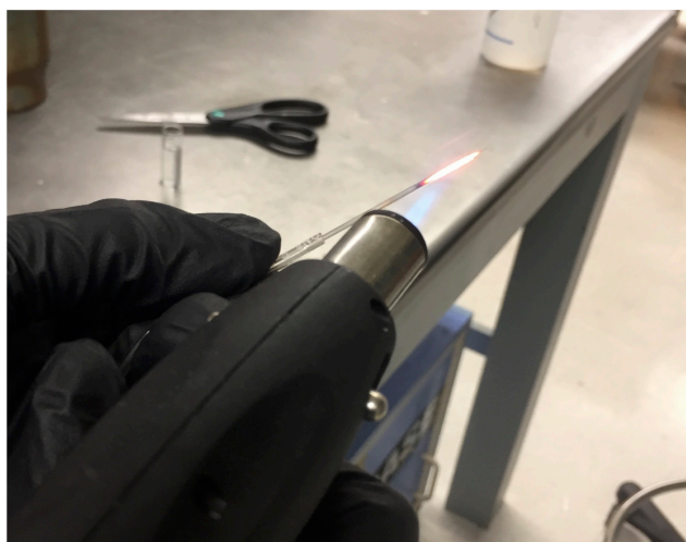
Figure A.5. Thermal Deposition of Pyrolytic Carbon in a Pulled Quartz Electrode. A handheld butane torch was used to gently heat the ethylene gas flowing inside the pulled capillary such that decomposition of the ethylene deposits thin layers of pyrolytic carbon.
