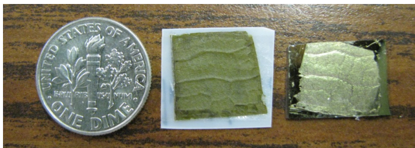
Figure 7.4. Photograph of a dime (left), an Aristolochia esperanzae leaf (middle), and corresponding pNBF8 coating of the leaf (right).
