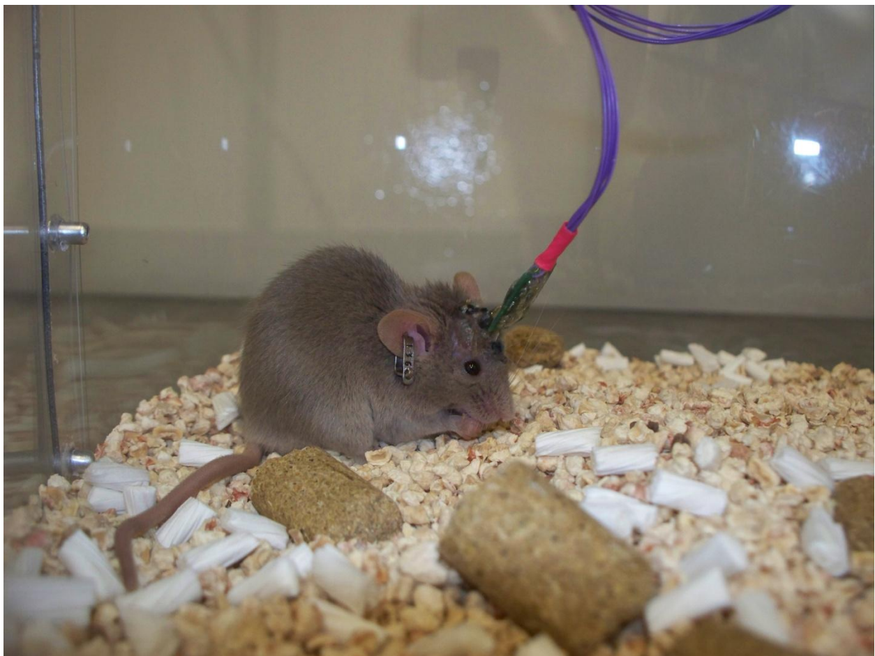
Figure 2-3: Picture of a post-operative mouse showing the implanted headmount connected to a preamplifier.
