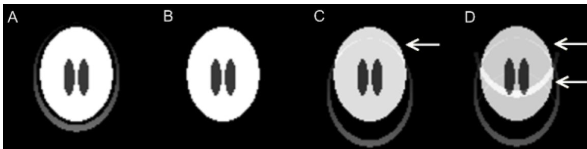
Figure A.3: The effects of incomplete fat saturation in EPI. In an inhomogeneous sample containing multiple tissue types, such as CSF (black), brain tissue (white), and subcutaneous fat (grey) (A), proper fat saturation completely suppresses the fat signal from images acquired with EPI (B). However, if fat saturation is incomplete in the EPI acquisition (C), the signal from fat is shifted along the phase encoding direction (vertically, in this case), corrupting voxels containing signal from other types of tissue (arrow). SENSE reconstruction artifacts can increase the number of corrupted voxels by causing ghosting of the artifacts into the center of the image (D).
