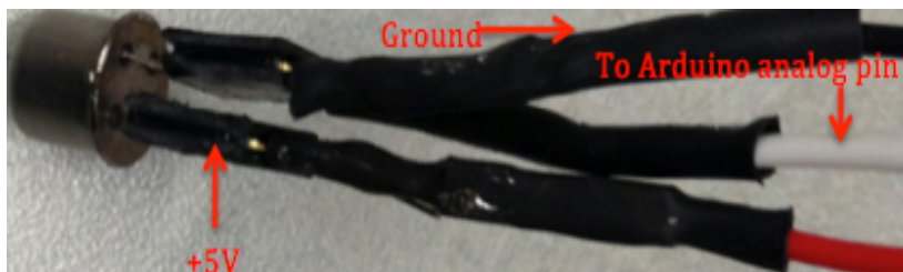
Figure 23. TGS 2620 Odor Sensor Data Logging Prototype Photo
