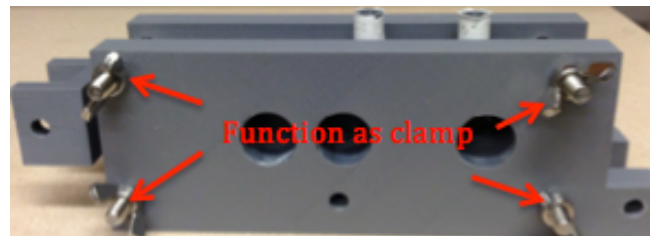
Figure 36. Assembled Real 3D Parts Object of LATTS. (A) A prototype photo of the LATTS for drosophilae training and testing. The main mechanical components of LATTS are composed of the 3D parts: a linear actuator and three quick connectors. The system is mounted on a wooden board. (B) Magnified illustrations showing the 3D parts and we call them together as base.
