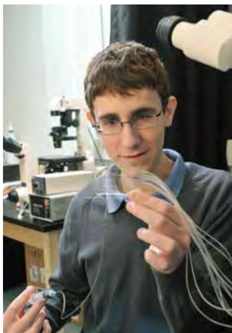
Will Matloff displays the 16-channel microformulator he has been developing in SyBBURE Searle. The device is designed to continuously formulate customized media mixtures at a rate of 500 nanoliters per minute.
