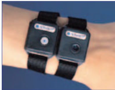
An actigraph, or movement sensor, measures movement and helps researchers track sleeping and waking patterns without doing sleep studies.
