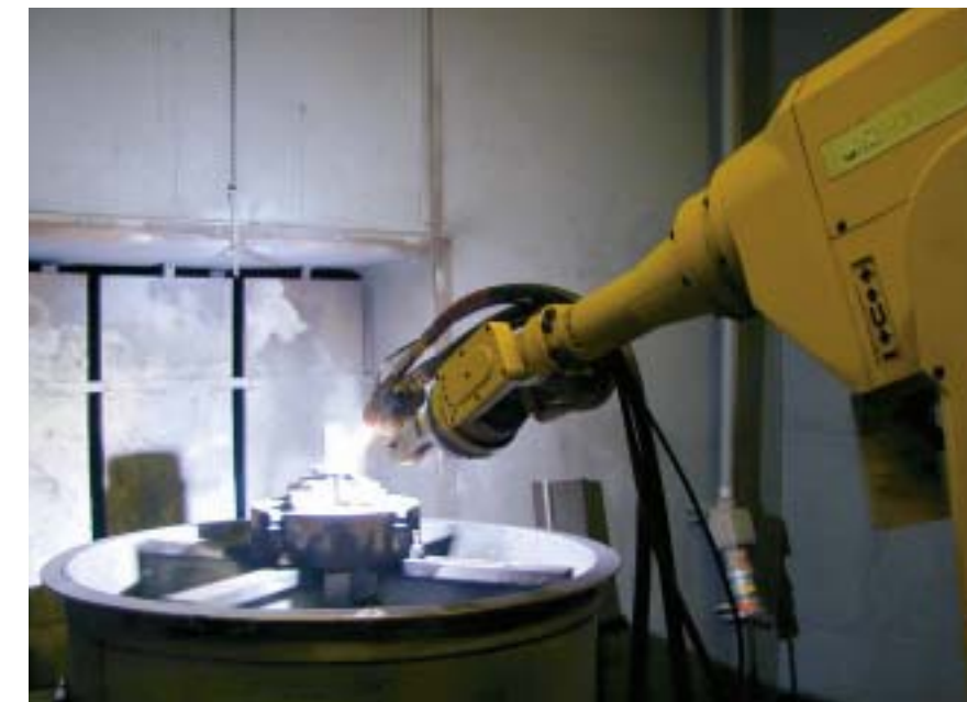
At Plasma Processes, a robot manipulates a plasma gun to deposit ceramic materials similar to those used to coat rocket engines.
