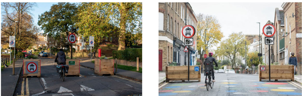
Figure 1.7: Modal filter that completely blocks car traffic (left) and a modal filter that is enforced by camera (right)
