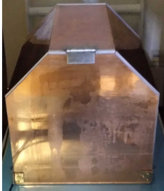
Figure 4.5: The copper-clad acrylic shielded box inside of the 47.5 mT low-field scanner.
