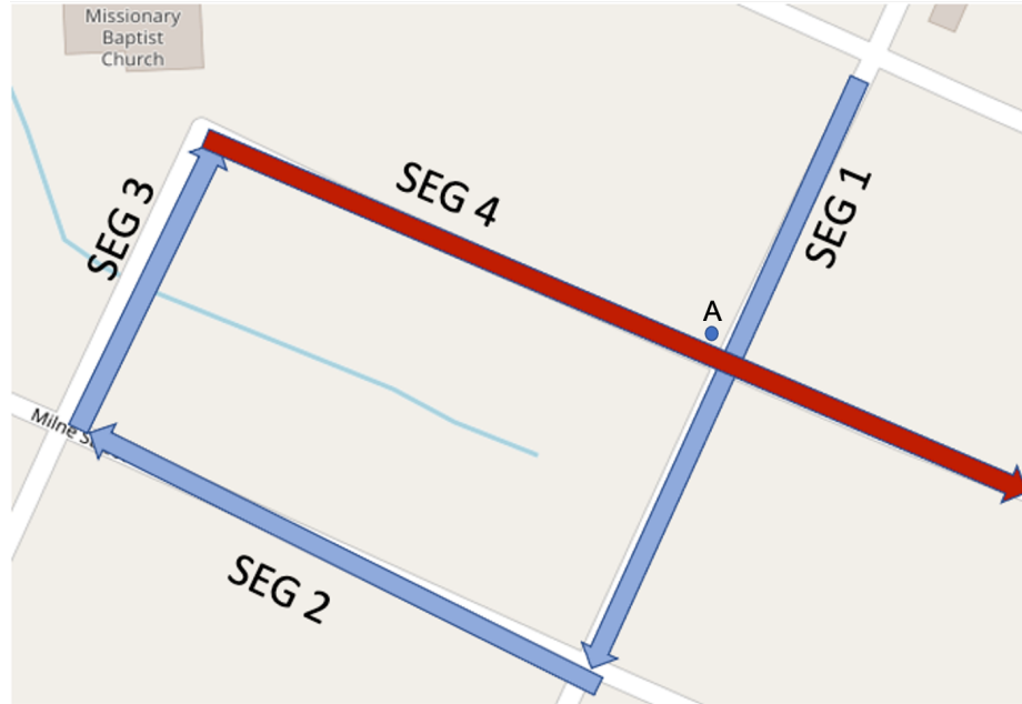
Figure 4.4: Overlapping segments. Segments 1 and 5 traverse the same section in opposite directions. Intersecting segments. Vehicle locations near the intersection of segments 1 and 4 can lead to incorrect mapping. Stops not shown.
