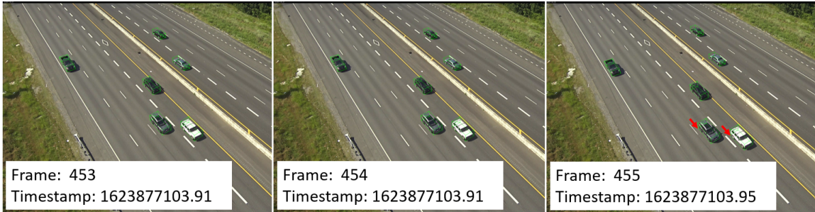
Figure J.10: Example of a doubled frame. Frame indices 453 and 454 for camera p1c2 in sequence 0 display identical frames and timestamps. The following frames shows object positional changes (red arrows) consistent with a larger time delta than is indicated by frame timestamps.
