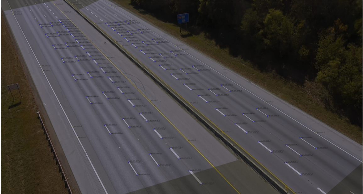
Figure O.13: Correspondence points (blue) and fields of view (shaded polygons) for each roadway direction of travel, labeled in a single camera field of view (P27C01). Around 100 correspondence points are visible for each side of the roadway.
