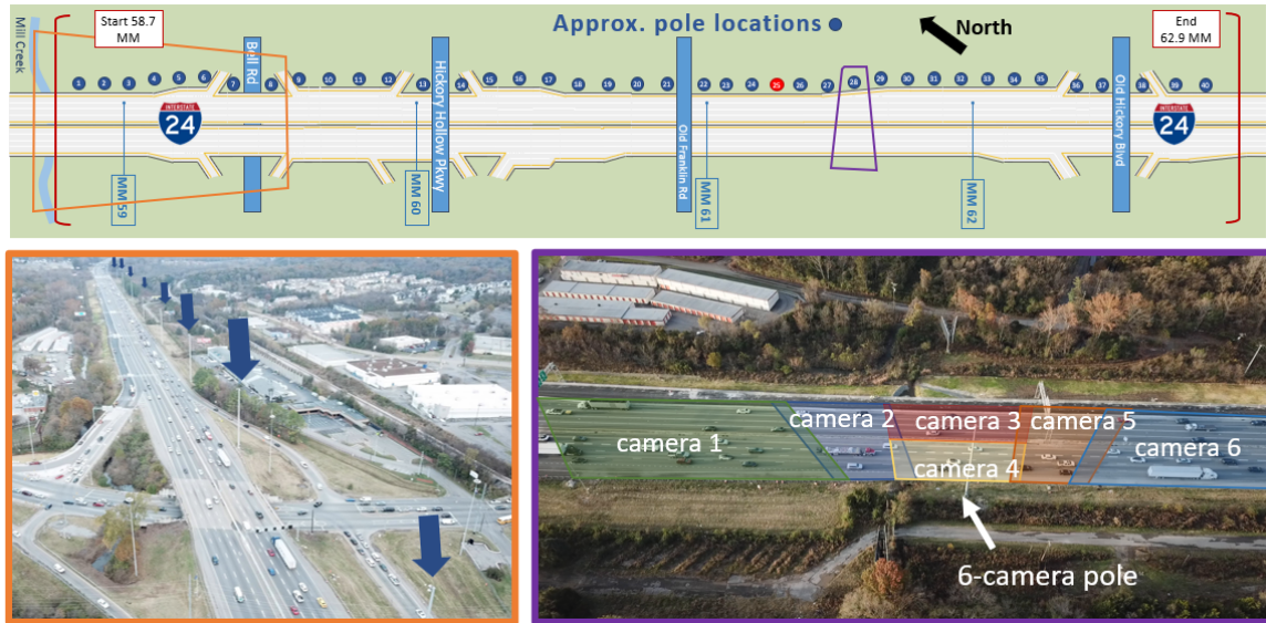
Figure 7.2: (top) Graphical overview of the I-24 MOTION system. Each blue dot represents a camera pole with 6 cameras. Red dot indicates a camera pole outage (Pole 25). (orange) drone image showing 8 of the 40 system camera poles. (purple) Typical 6 camera per pole coverage layout. Best viewed zoomed-in.
