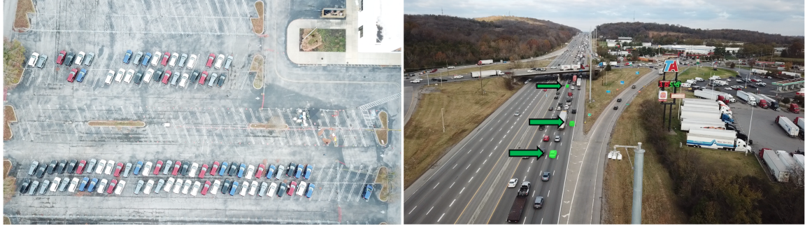
Figure 8.1: (left) The fleet of instrumented vehicles used to execute control strategies during the CIRCLES 2022 experiment. (right) Software-controlled instrumented vehicles (green) are visible on the roadway, and their positional data is recorded by I-24 MOTION cameras. (Drone imagery courtesy of Said ElSaid).
