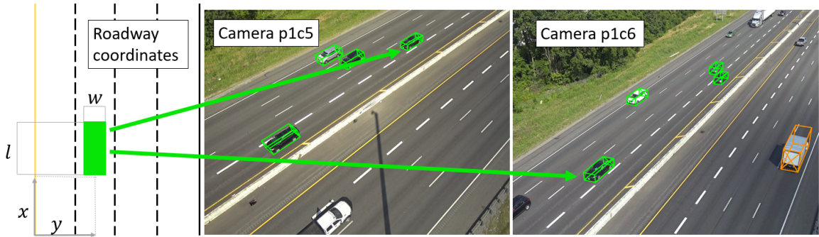
Figure 6.2: Example single annotation. The annotation is stored in roadway coordinates (left) but can be projected into cameras 5 and 6 on pole 1 (p1c5 and p1c6).
