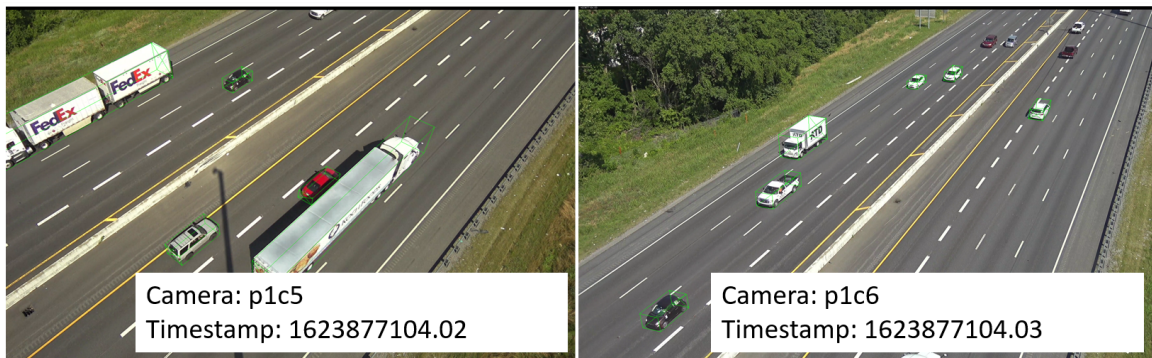
Figure J.7: Example of phase and clock offset error. Closest reported timestamps from cameras are unequal (phase), and the positions of vehicles in camera p1c5 suggest this frame was recorded later than p1c5 (clock offset).
