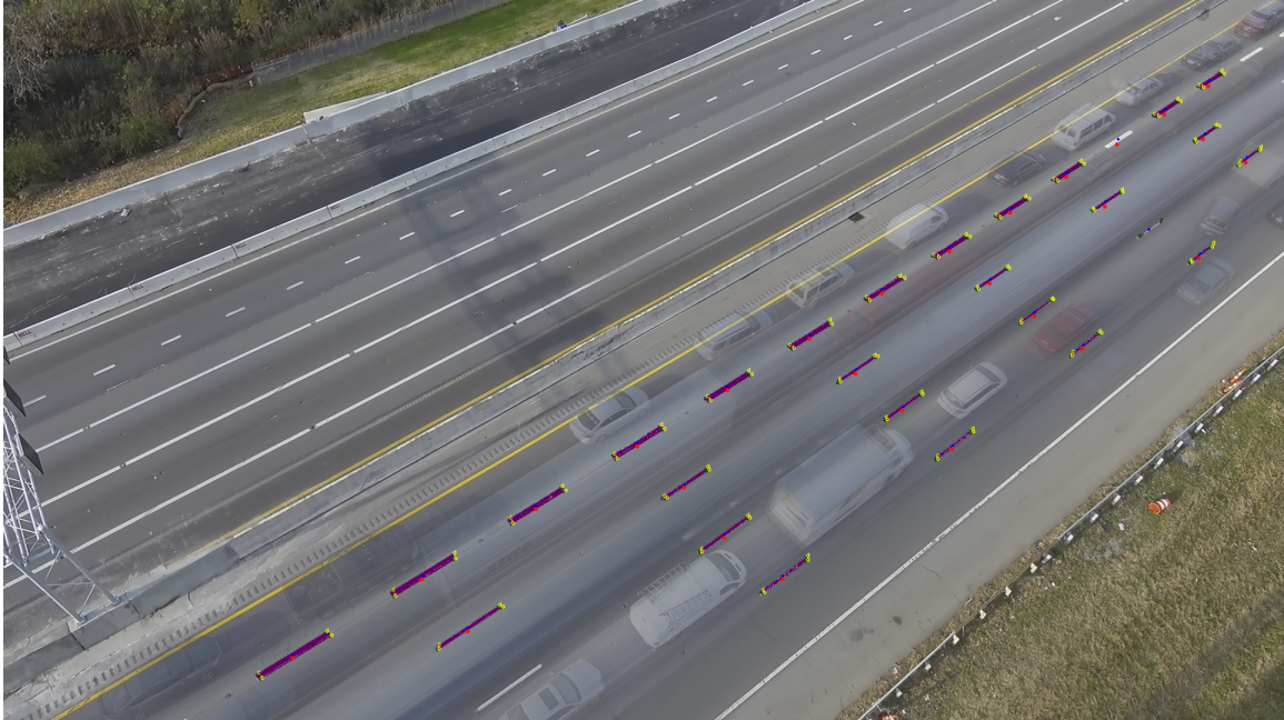
Figure P.19: An example of SIFT-FLANN based seed points from step 6 (red dots), detected contours (purple outlines) and re-detected dash corner points (yellow dots) for a 1-minute average frame. Because traffic at this time instance was partially stopped, some vehicle artifacts are visible in the averaged frame. A few dashes are not successfully rediscovered. Credit: Gergely Zachar.
