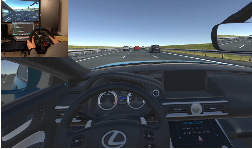
Figure 5.4: Naturalistic driving in a car-following scenario with a gaming laptop, a Logitech racing wheel, and the Unity game engine.
