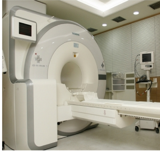
Figure 2.4: A 1.5T MRI scanner (Park et al., 2014). The images acquired are under creative common license.
