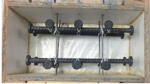
Figure 58: Plan view of two-directional rebar reinforcement (with ties) for the alkali-boosted bidirectionally reinforced concrete specimen.
