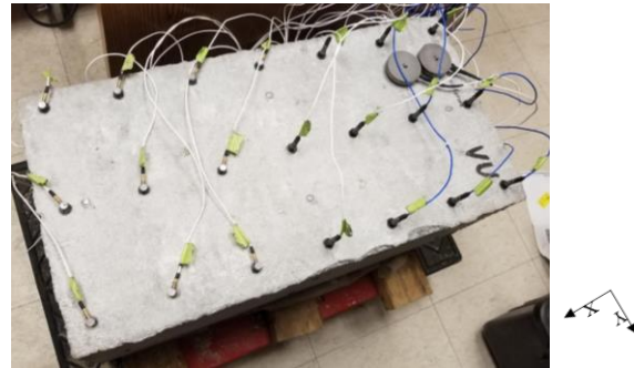
Figure 53: Locations of accelerometers and pumping and probing excitation actuators on the surface of the validation specimens: (a) diagram of the surface of the specimens with all 21 sensors tables, and all 10 pumping and probing excitation actuator locations; (b) experimental setup on the surface of the specimen for pumping and probing excitation actuator location 8.
