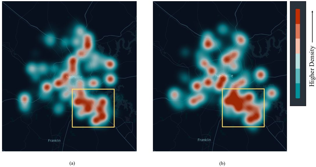
Figure 3.9: Batch Model (a) vs Streaming Model (b): These predicted heatmaps demonstrate that the streaming model adjusts more quickly to new incident distributions. Starting with a survival model learned from the training set, we fed the models synthetic incident data with incidents only occurring in the yellow boxed area, which means that the model should learn that there is now a higher incident likelihood in this area. The batch model picks up the new pattern weakly, whereas the streaming model shows higher likelihood in marked box.
