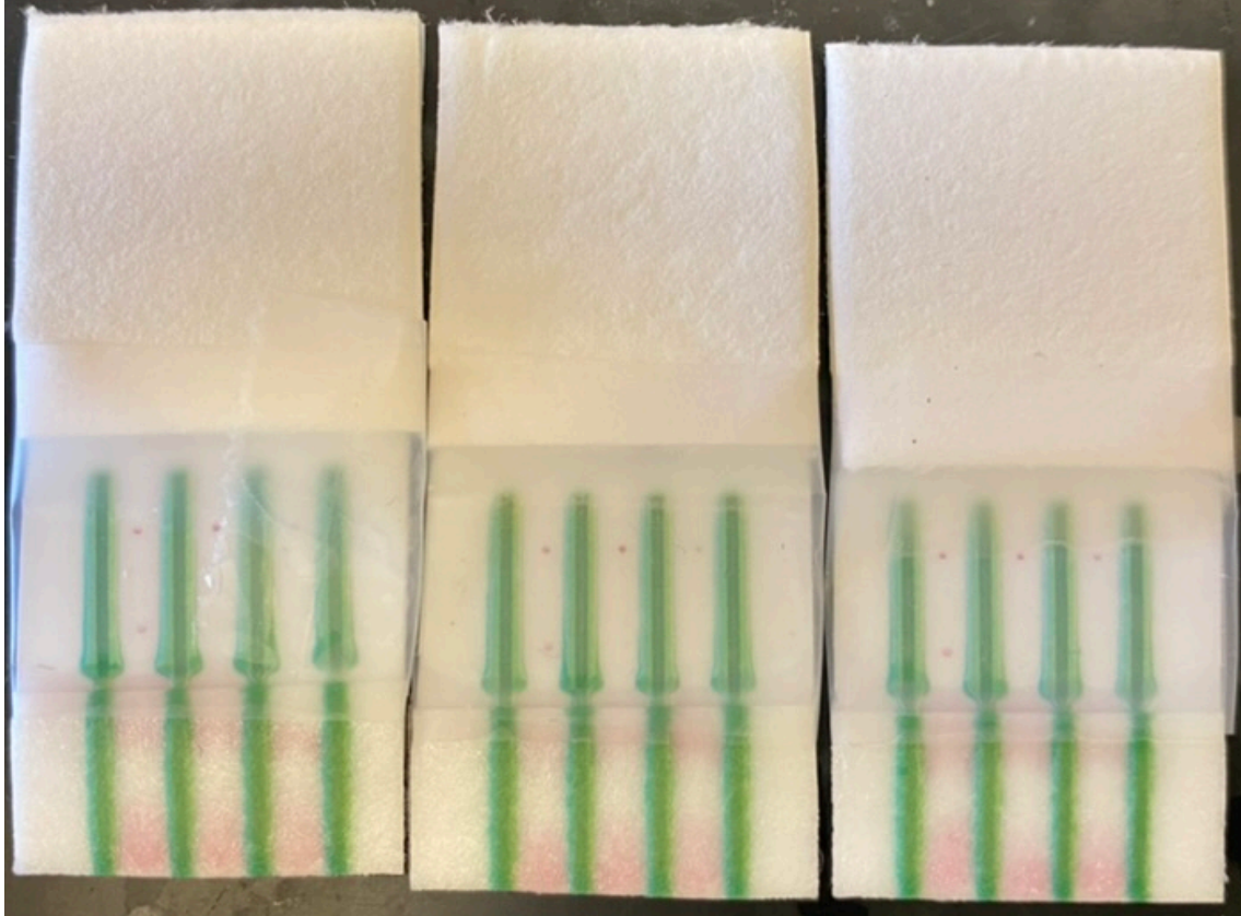
Figure 32. Dipstick assays run in triplicate with each channel corresponding (left to right) to detection of CRP, PCT, and HRP2.
