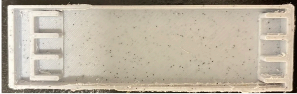
Figure 33. Custom 3D printed cassette that fits three single LFAs.
