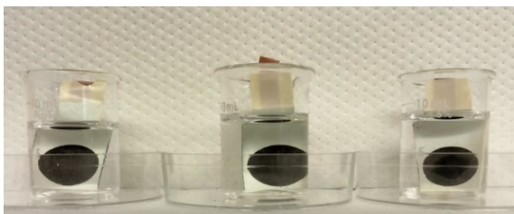
Figure A.3: Acid treatment of electrodes in 0.05M H 2 SO 4 for 48 hours
