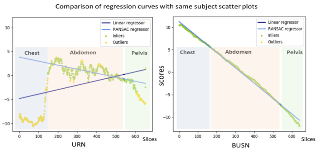
Figure 2.4: A representative subject was evaluated with URN (left) and BUSN (right). Green scatters are inliers of influence to the regression, yellow scatters are outliers of no influence to the distributed data. Darker blue line indicates the normal linear regression on scatters points, lighter blue line is the RANSAC regressor result according to inliers. Left panel presents the single URN regression with amounts of outliers result in failure of linearity nature in chest and pelvis regions. Right panel shows the testing result of BUSN method, the distributed scores follows good linearity in chest, abdomen and pelvis regions in CT scan. In summary, BUSN takes advantage of self-supervised network, which presents better continuity in regression result among neighbor slices and shows scatter plots without number of outliers.
