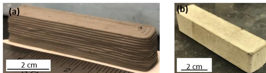
Figure 5-1. Flexural testing beams (a) cast, and (b) 3D printed with a concentric pattern
