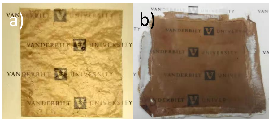
Figure 3.18: Photographs of a composite a) cPPSA-PPSU dual-fiber membrane and b) cPPSA-PPSU pore-filled membrane.
