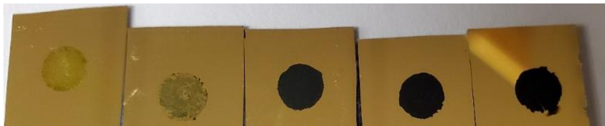
Figure 5.1: PSI multilayer films after polymerization of PPy. From left to right, the amount of charge passed was 0, 1, 5, 10, 15 mC total or 0, 14, 70, 140, and 210 mC/cm 2 .
