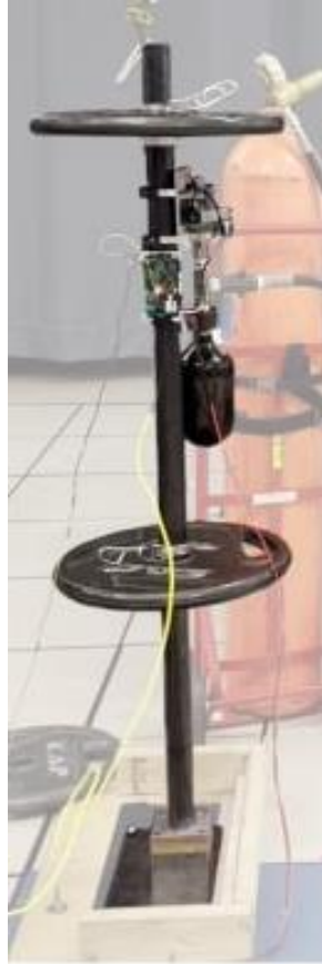
Figure 4-2. The rocking block experimental apparatus v2 with the CGT v2 attached.
