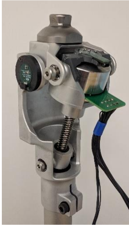
Figure 2-1. Swing-assist knee prosthesis prototype (shown without embedded system or battery).
