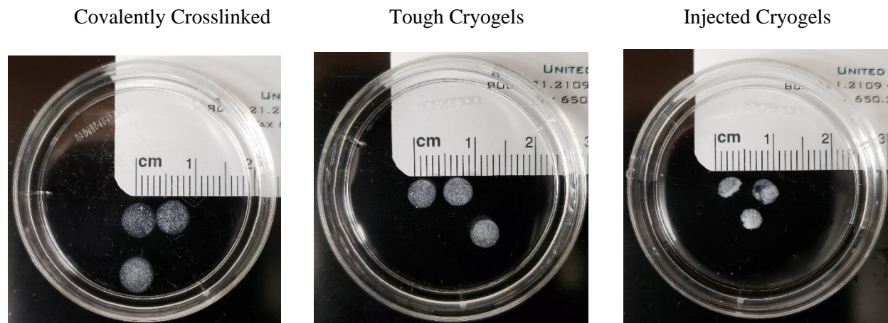
Supplemental Figure 4.S2: Pictures of cryogels in DI water (Covalently Crosslinked), in CaCl 2 (Tough Cryogels), and after injection through a 16G syringe (Injected Cryogels).
