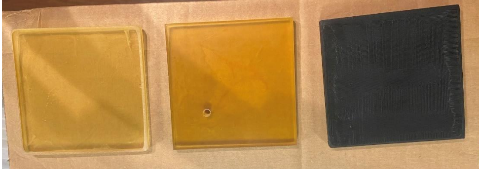
Figure 3.1: Samples used in testing (from left to right: epoxy, epoxy with hole, and ABS)
